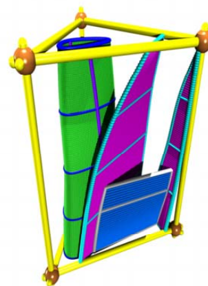
Figure 3. Prism representation of the temperature variation of the ternary phase diagram for a mixture of saturated and unsaturated lipids and cholesterol. [27]
