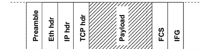
Figure 7: Frame and payload.
