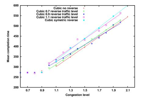
Figure 9: Impact of reverse traffic level on mean completion time for CUBIC, 19.8 ms RTT
