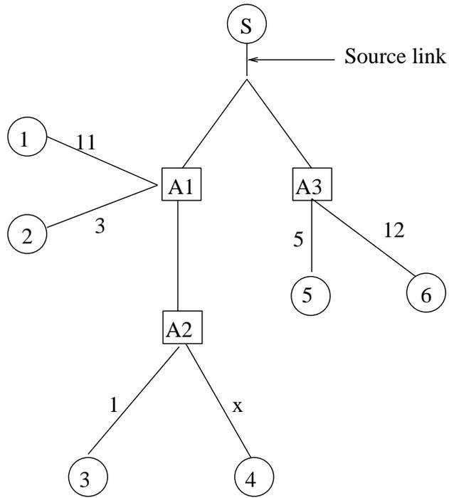
FIG. 4 – Example with a hierarchy of routers
