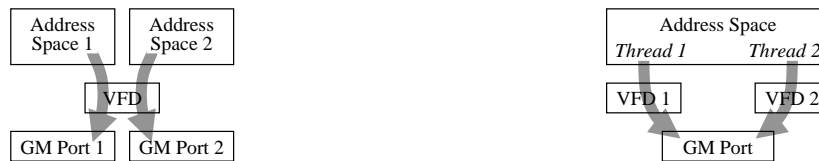
(a) Different address spaces use different GM ports even for the same descriptor.
