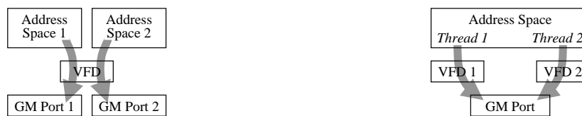
(a) Different address spaces use different GM ports even for the same descriptor.
