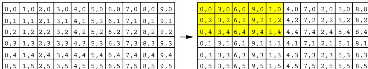
Figure 7: A  $10 \times 6$  grid of virtual processors is mapped onto a  $2 \times 2$  grid of physical processors. The dataflow matrix is  $T = L.U$ . Processor  $(0,0)$  is shaded to show the distribution over physical processors.
