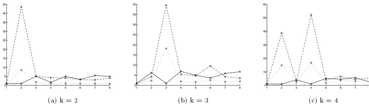
Figure 8: These graphs represent the ratio of the communication time for a  $U$  matrix with standard distribution schemes over the time using the grouped partition scheme. For each graph, the dotted line is the ratio of the **CYCLIC(20)** distribution over the grouped partition, the dashed line is the ratio of the full **BLOCK** distribution over the grouped partition, the solid line is the ratio of the **CYCLIC** distribution over the grouped partition.
