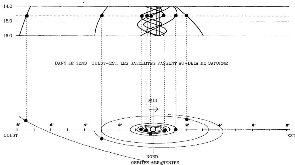
The distances  $\Delta\alpha \cos \delta$ , measured on the curves for the chosen date, are plotted in abscissa on west-east axis. The ordinate is given by the apparent orbits. The direction of the rotation indicates if the satellite is before or behind the planet on its orbit.
