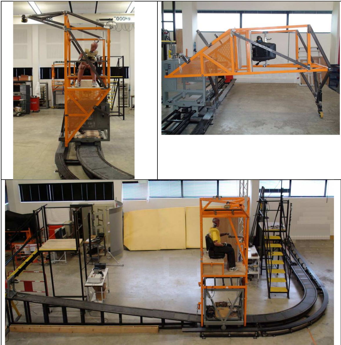
Figure 1: test bench for generating the conditions of a full tip-over of the replica of a commercial cab.
