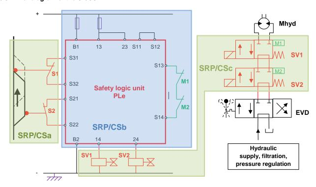
Figure 25: Final diagram of the SF/CS
