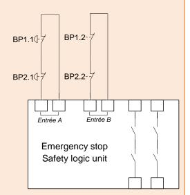
When the manufacturer of the safety logic unit foresees the possibility of connecting several input elements in series, the corresponding DC value must be indicated as a function of the number of expected input components.
