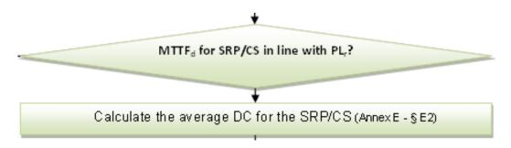
Extract from Graph 2: Details of the design of an SRP/CS to achieve a required PL
