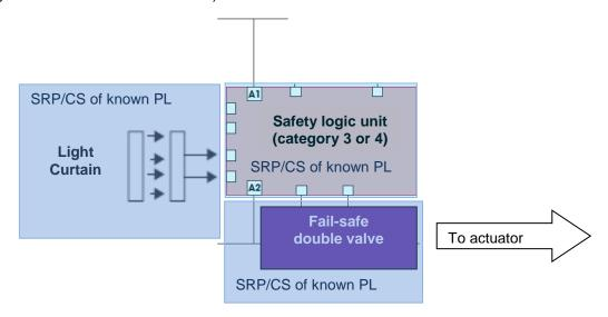
Figure 4: Example of a SF/CS composed of 3 SRP/CS of known PL
