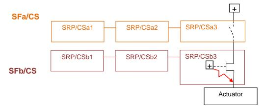
Figure 9: Example of failure of an electronic output
