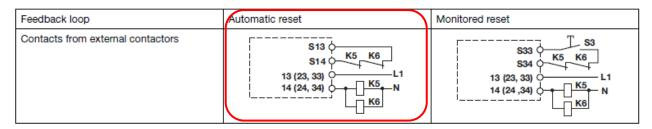
Figure 18: Extract from the manufacturer's instructions for the safety logic unit
