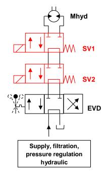
Figure 21: Diagram of the hydraulics to be implemented
