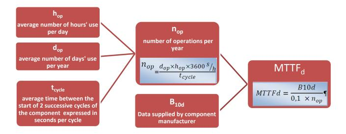
Figure 7: Calculating the MTTF<sub>d</sub> for a single component based on its B<sub>10d</sub>
