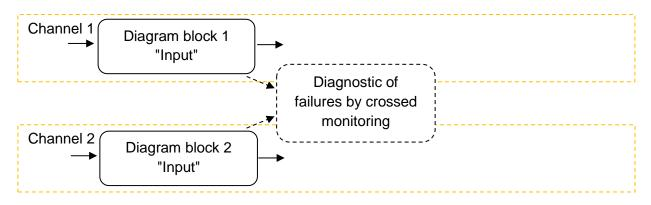
Figure 13: Breakdown of SRP/CSa with block diagrams
