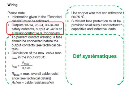
Figure 17: Extract from the manufacturer's instructions for the safety logic unit
