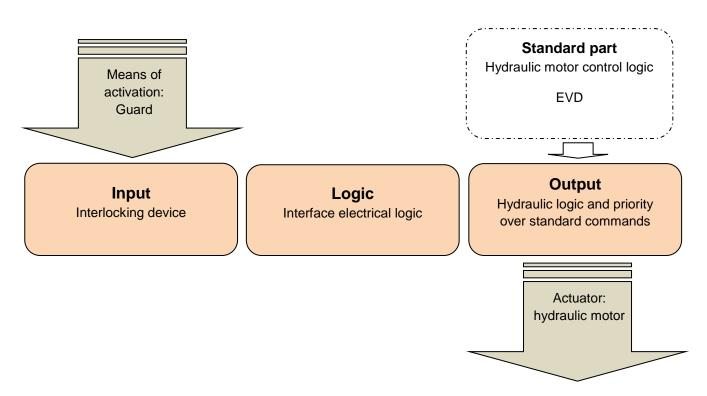
Figure 11: Basic logical structure for the SC/FS
