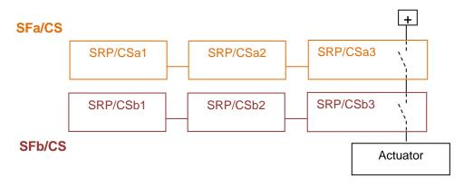
Figure 8: The signal from SFa/CS to the actuator passes through SRP/CSb3, which is an element of SFb/CS
