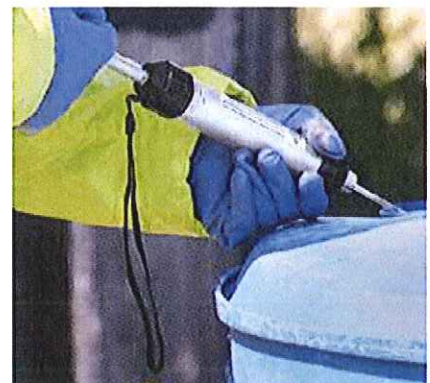
First responder uses RAE Systems colorimetric tubes and hand pump to measure VOC levels inside a barrel
