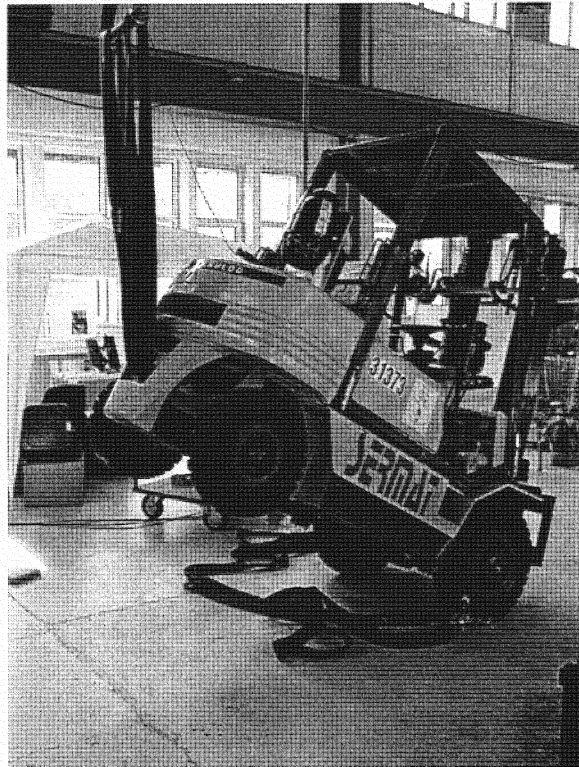
Figure I- 5 : View of the measurement of the height of the center of mass by rotating around the pitch axis
