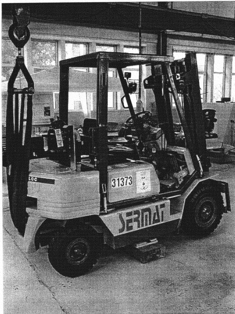
Figure I- 3 : View of the measurement of the longitudinal position of the center of mass
