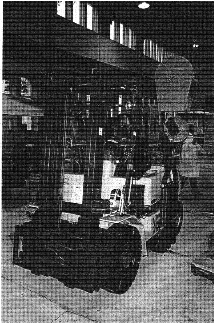
Figure I- 12 : Measurement of roll inertia by free oscillations.
