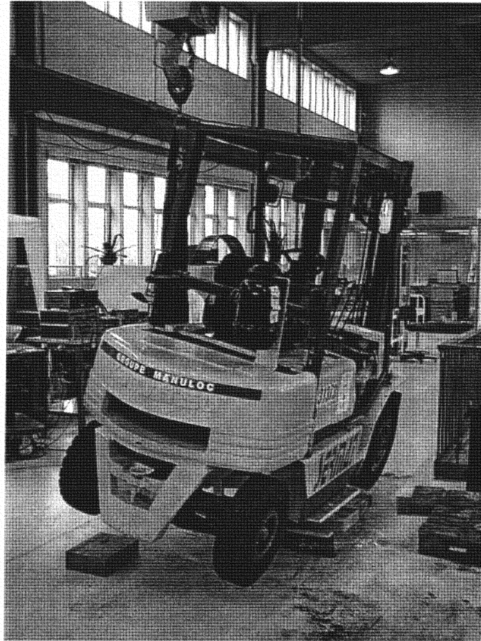
Figure I- 8 : View of the measurement of the height of the center of mass by rotating around the roll axis
